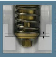
Safety Pressure Relief: Under normal pressure, the valve stays closed, directing the hot fluid to be cooled by the heat exchanger. Excessive pressure pushes up on the valve, compressing the spring and allowing fluid to flow straight out of the system without being directed by the heat exchanger. When the valve is closed, it sits at the bottom line. Excessive pressure pushes the spring to move the valve to the upper position pictured in the diagram.
