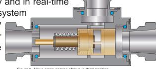
Figure 2. Valve cross-section shown in "hot" position
