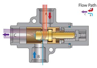
Fig1: Restricted cold flow into port B
